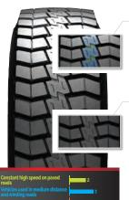
Centre block & Tie-bar - Stable centre block to minimise tread damage off road
