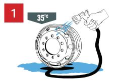
Allow the wheels to cool below 35°C, then remove the nut covers. Rinse with clean water to avoid scratches and corrosion, and ideally, use a high-pressure washer.
