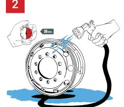
In order to avoid scratches and corrosion, the wheels should be washed with clean water.
